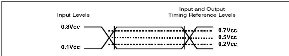
Figure 52. AC Measurement I/O Waveform
